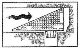
Place the WEDGE in the gutter with the oval ring in the downspout opening, pointing with sloped end facing the oncoming water.
